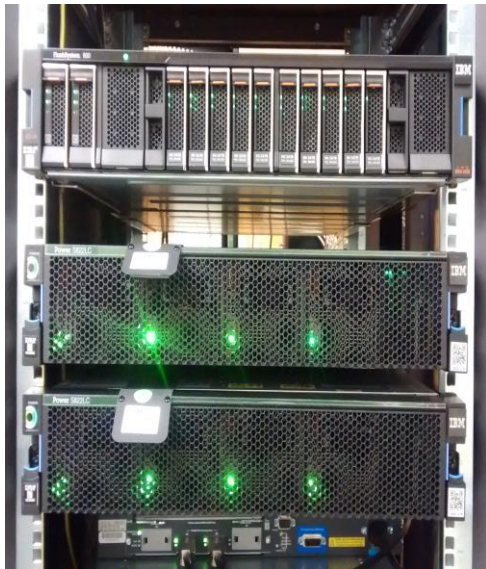
The TWO IBM S822LC power nodes and the IBM Flash System 900 machines at CHMPR
